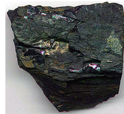
Laminated Castile Formation basinal evaporites. Dark laminae are calcite plus organic matter; light laminae are gypsum (Peter Scholle)
