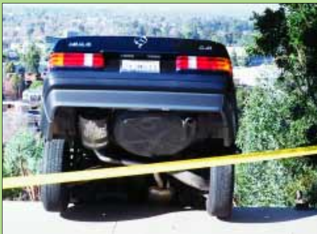
◆ FIGURE 1 This luxury car seems to be pursuing the garage in which it is normally kept. The house and garage slid down the hillside, but the car was parked with its rear wheels on the driveway, which was on stable ground. Nobody was hurt; Northridge, 1994
