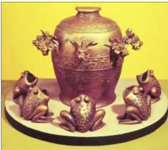
◆ FIGURE 4.6 The first earthquake detector, invented about A.D. 130 by Chinese scholar Chang Heng. Balls held in the dragons' mouths were aligned with a pendulum inside the vase. When an earthquake occurred the pendulum swung and pushed balls into the mouths of the frogs aligned with the pendulum's swing. If the frogs facing north and south contained balls, for example, Chang Heng could say that the earthquake epicenter was north or south of the instrument.
