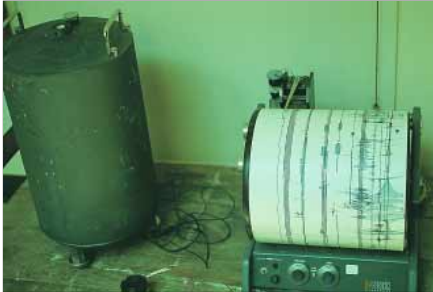
◆ FIGURE 4.5 Seismometer ( left ) and seismogram ( right ) used to demonstrate method of detecting and recording earthquakes. The record on the seismogram is not an earthquake, but represents the seismometer's detection of vibrations from students' footsteps amplified about 2,000 times.
