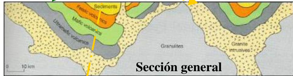
FIGURE 6-22 Generalized cross-section through two greenstone belts. Note their synclinal form and the sequence of rock types from ultrabasic near the bottom to felsic near the top. A late event in the history of the belt is the intrusion of granites. Ultramafic basal layers are particularly characteristic of greenstone belts in Australia and South Africa but do not occur in the Archean of Canada.
