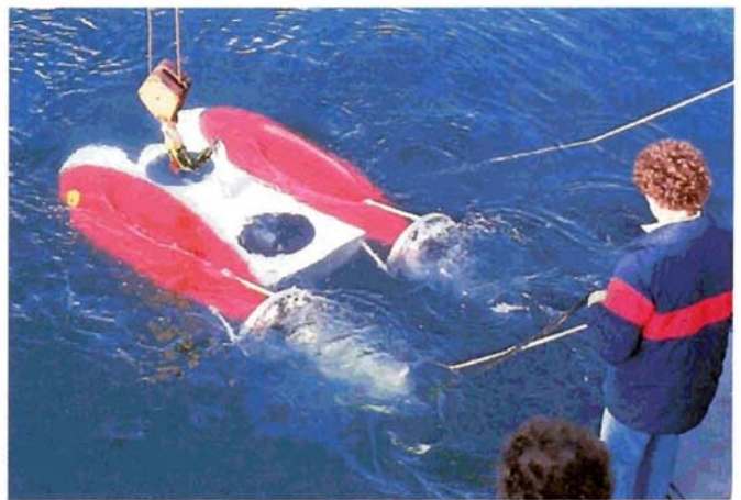
FIGURE 17.21 The Benthic Explorer . This small robotic vehicle can explore the seafloor while being directed from shipboard. (T. Kleindinst/Woods Hole Oceanographic Institution.)
