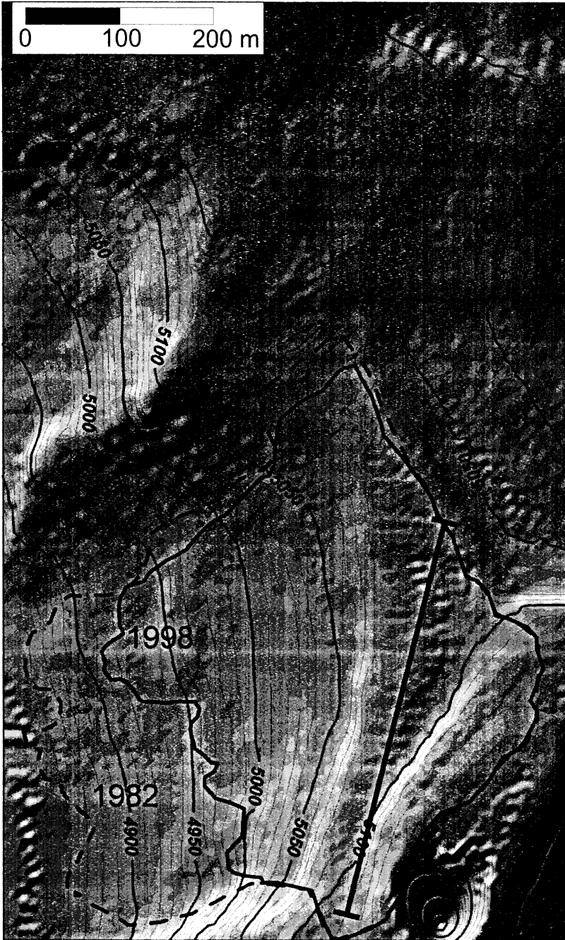
Fig. 2. DEM of Iztaccíhuatl volcano showing the extent of Ayoloco glacier in 1982 and 1998 (dashed and solid line, respectively). The GPR profile location is indicated with a black line, and the dotted area is the diffuse-degassing field.
