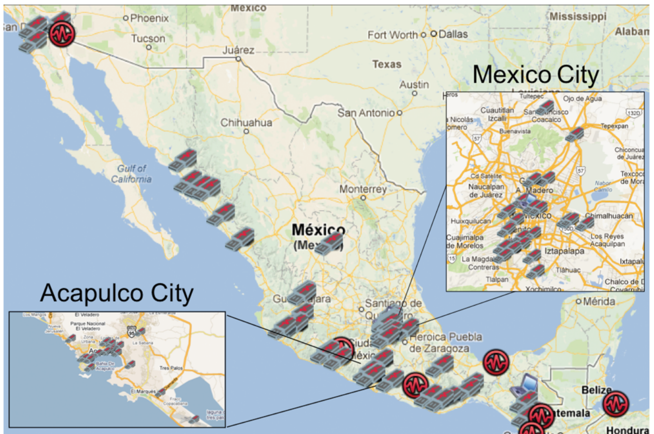
▲ Figure 1. Distribution of sensors in Mexico (April 2013). USB-like icons indicate external sensors. Laptop-like icons show internal sensors. Circles correspond to earthquakes M_w > 3.5 as reported by the U.S. Geological Survey (USGS).
