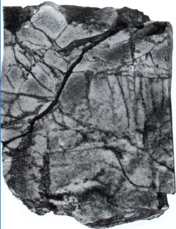
FIGURE 6.5 Fractured core of Gargaf Group sandstone (Cambro-Ordovician)
