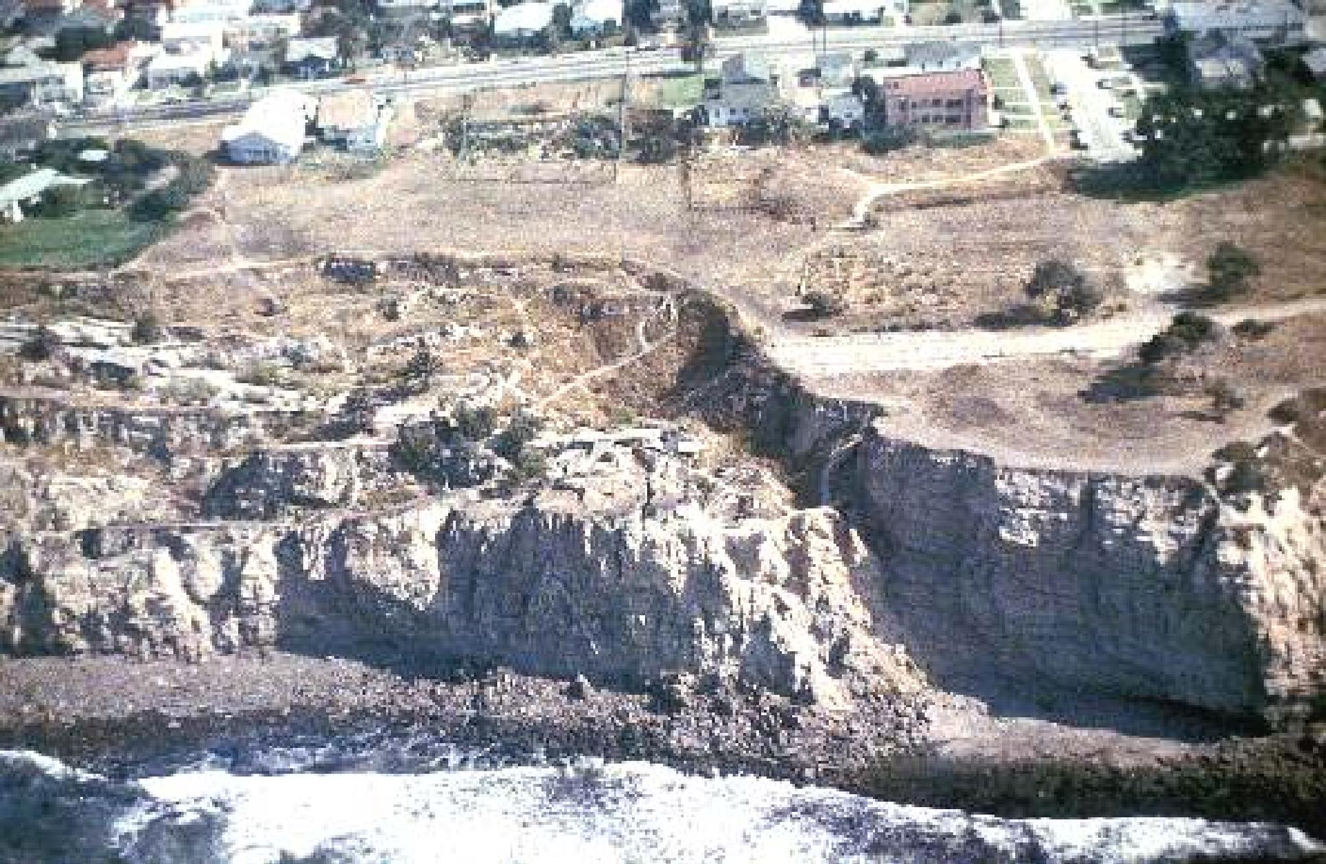
The road to nowhere was truncated by the Portuguese Bend landslide that became active in 1956. The damages that it caused to homes in that area led to a precedent-setting, class-action suit against the County of Los Angeles. The landslide is due to the failure of Tertiary silt when subjected to wave action at its base.
