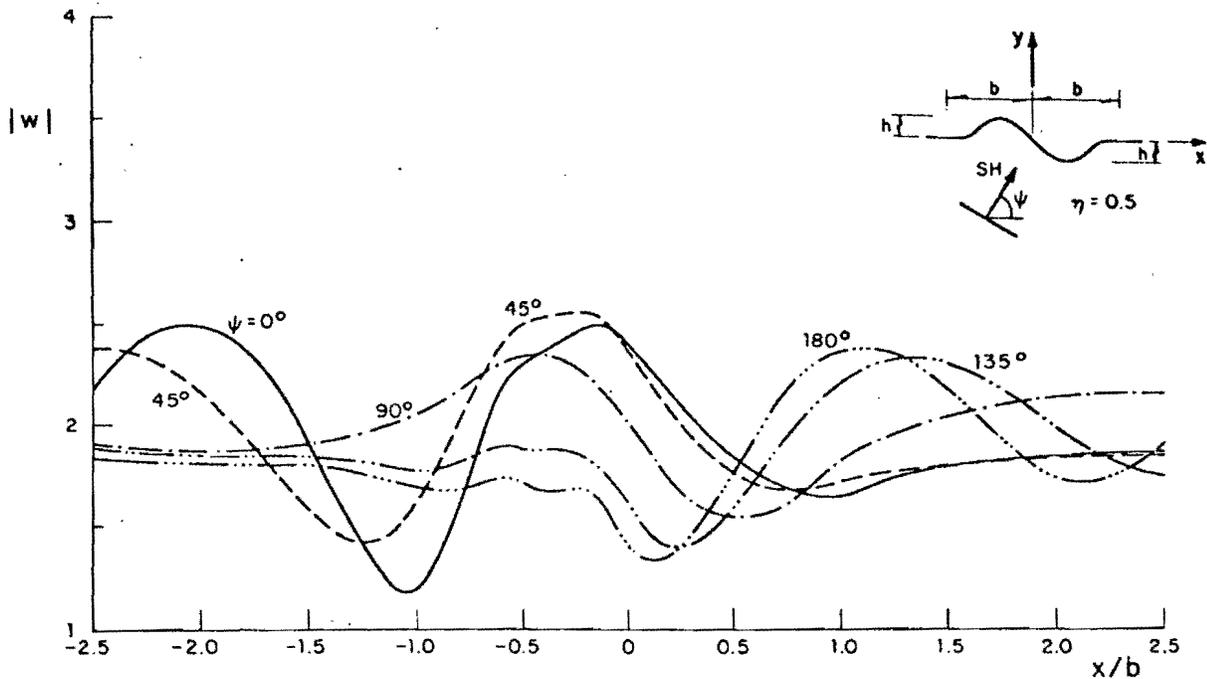
FIG. 7. Displacement amplitudes on the surface of the mixed topography with  $h/b = 0.25$  for the five incidence angles and normalized frequency  $\eta = 0.5$ .
