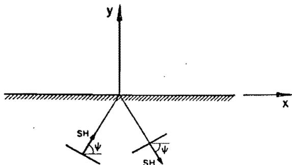
FIG. 4. Incident and reflected SH plane waves.
