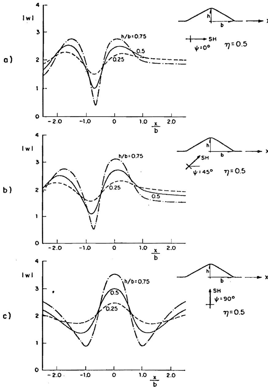
FIG. 6. Displacement amplitudes on the surface of ridges with different aspect ratios and three incidence angles. Normalized frequency  $\eta = 0.5$ .
