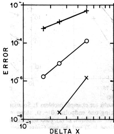
Fig. 3. Convergence results for example problem 2, using Gauss points to define piecewise constant (+ - +, slope = 2), piecewise linear (o - o, slope = 4), and piecewise quadratic (x - x, slope = 6) interpolation for the variable coefficients.
