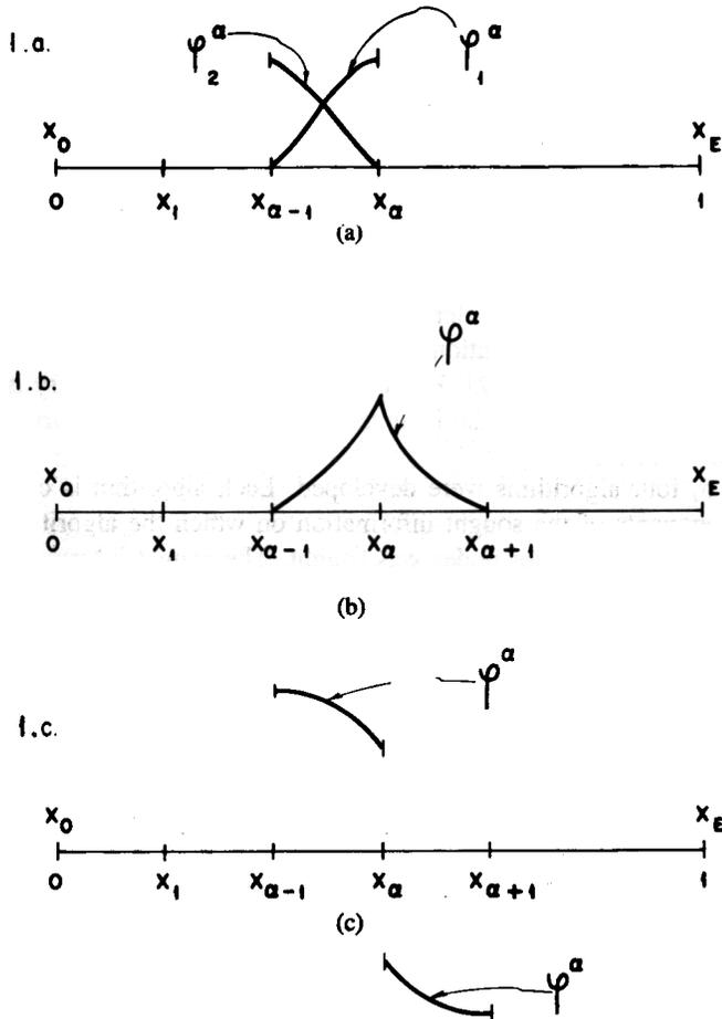
Fig. Test functions. (a) Algorithm 1, (b) Algorithm 2, and (c) Algorithm 3.
