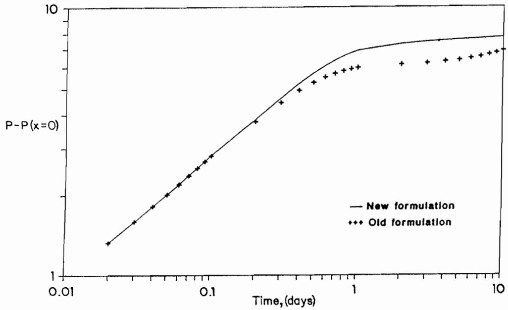
Figure 5: Comparison on pressure drop behavior for new and old formulations.
