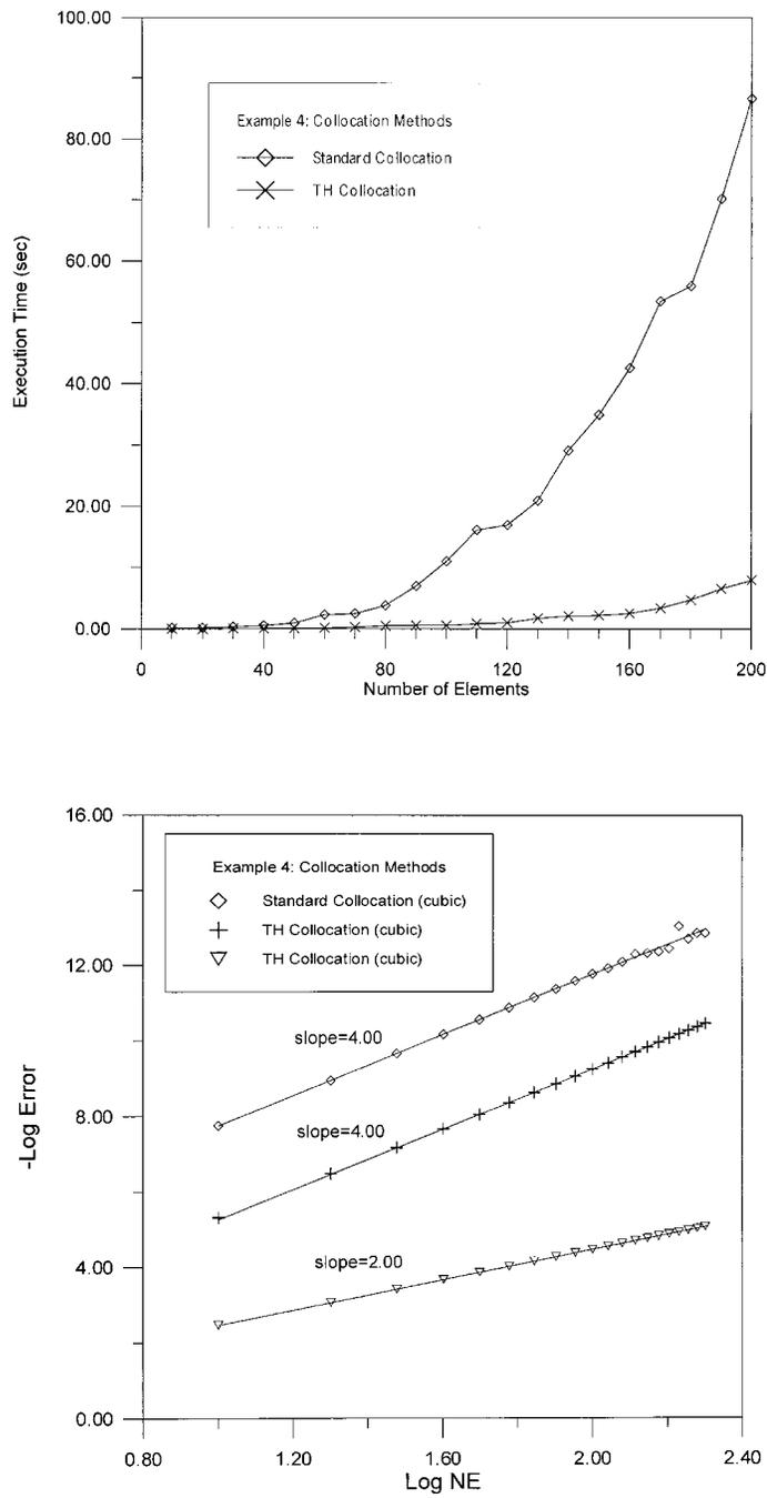
FIG. 5. (a) Example 4. Performance comparison between Standard and Trefftz–Herrera collocation. (b) Example 4: Convergence rate of Trefftz–Herrera collocation method using cubic and quadratic weighting functions comparing to Standard Collocation Method using cubic weighting functions.
