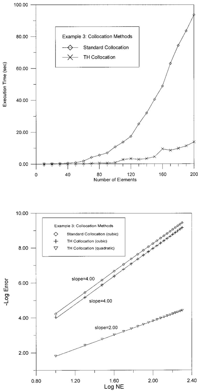
FIG. 4. (a) Example 3. Performance comparison between Standard and Trefftz–Herrera collocation. (b) Example 3: Convergence rate of Trefftz–Herrera collocation method using cubic and quadratic weighting functions comparing to Standard Collocation Method using cubic weighting functions.
