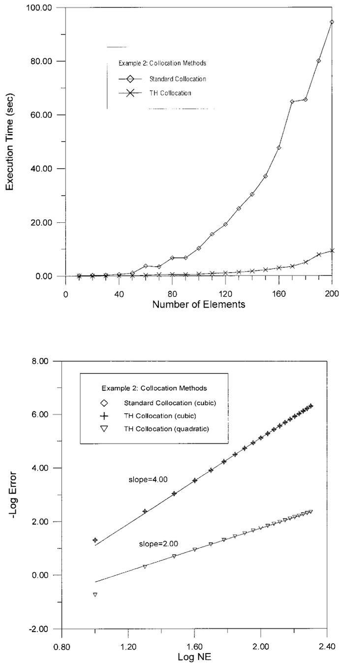
FIG. 3. (a) Example 2. Performance comparison between Standard and Trefftz–Herrera collocation. (b) Example 2: Convergence rate of Trefftz–Herrera collocation method using cubic and quadratic weighting functions comparing to Standard Collocation Method using cubic weighting functions.
