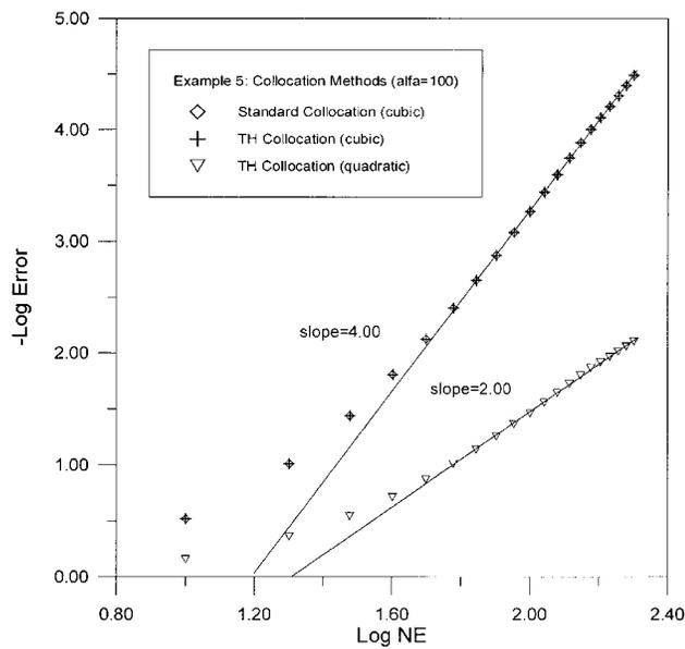
FIG. 7. (c) Example 5: Convergence rate of Trefftz–Herrera collocation method using cubic and quadratic weighting functions comparing to Standard Collocation Method using cubic weighting functions (Case  $\alpha = 20$ ). (d) Example 5: Convergence rate of Trefftz–Herrera collocation method using cubic and quadratic weighting functions comparing to Standard Collocation Method using cubic weighting functions (Case  $\alpha = 100$ ).
