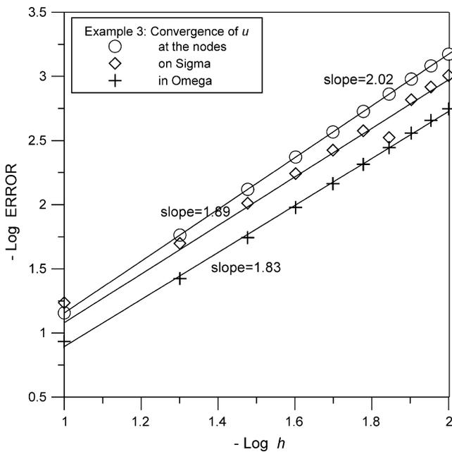
Fig. 7. Example 3: convergence rate of Trefftz–Herrera collocation method using linear weighting functions.
