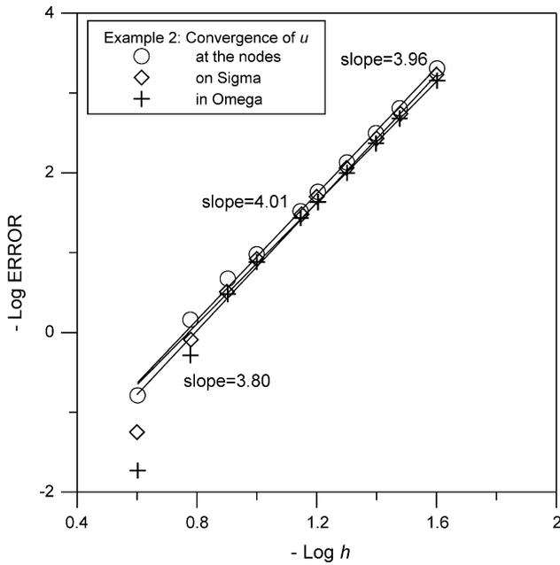
Fig. 6. Example 2: convergence rate of Trefftz–Herrera collocation method using cubic weighting functions.
