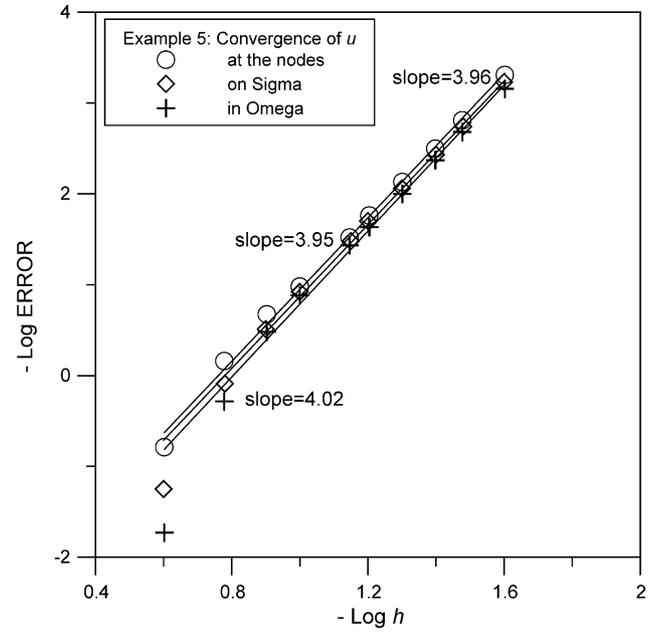
Fig. 12. Example 5: convergence rate of Trefftz–Herrera collocation method using cubic weighting functions.
