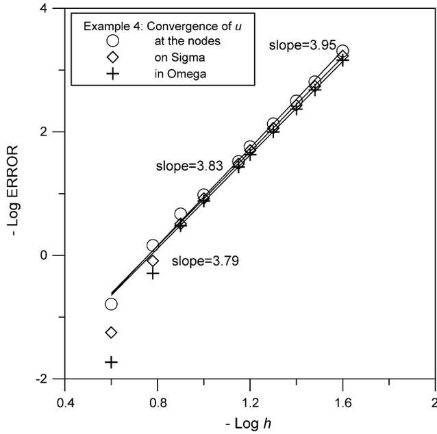
Fig. 10. Example 4: convergence rate of Trefftz–Herrera collocation method using cubic weighting functions.
