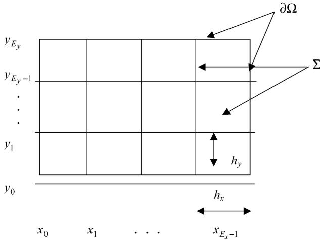
Fig. 1. Partition of the domain  $\Omega = [x_{\min}, x_{\max}] \times [y_{\min}, y_{\max}]$  in rectangular  $E_x \times E_y$  elements, where  $h_x = x_i - x_{i-1}$ ;  $i = 1, \dots, E_x$  and  $h_y = y_j - y_{j-1}$ ;  $j = 1, \dots, E_y$ .
