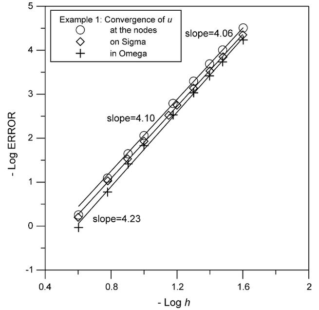
Fig. 4. Example 1: convergence rate of Trefftz–Herrera collocation method using cubic weighting functions.
