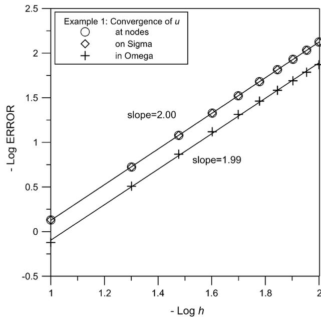
Fig. 3. Example 1: convergence rate of Trefftz–Herrera collocation method using linear weighting functions.
