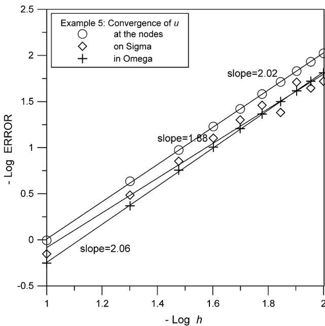
Fig. 11. Example 5: convergence rate of Trefftz–Herrera collocation method using linear weighting functions.
